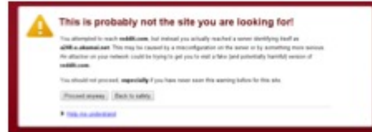
Figure 3: SSL warning for Google Chrome. The first paragraph changes depending on the specific SSL error.
